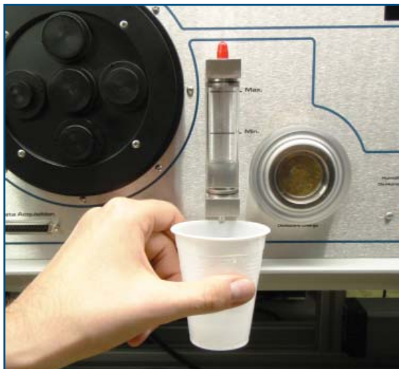
Figure 6 Emptying the Water Reservoir
