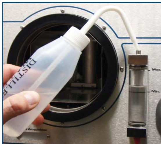
Figure 5 Filling the Water Reservoir
